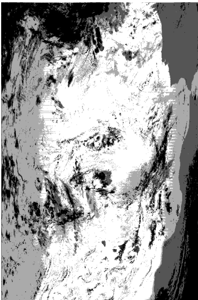
Fig. 3. MODIS segmented image with 4 segments. Input: 9-dimensional multiband image. Motivating choice of number of segments is the relative maximum value in the plot of Fig. 2.
