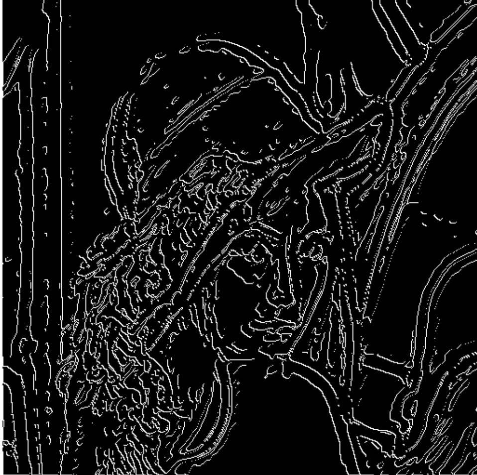
Figure 7. Edge map derived from Fig. 5 by subtracting the image from an eroded version of it: see text for details.
